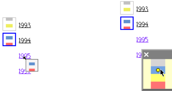
Fig. 4. Left: By default, a mouse click in a menu updates the scenarios shown in the menu’s currently highlighted marker. Here the marker for 1994 is highlighted (shown by its dark blue outline, and replicated in the mouse pointer), so a click on 1995 would switch the two 1994 scenarios to that value. The user can highlight a different marker by clicking on it. Right: Clicking and holding the mouse button on a menu item creates a pop-up that lets the user choose a single scenario to receive the clicked value. Here the user has clicked on 1996; releasing the mouse in its present position would set the year to 1996 in just the second scenario.
